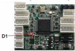
1.2 If D1 on sensor hub PCB is a diode, then upgrade is required, and C35 needs to be removed before you start upgrade steps below.
