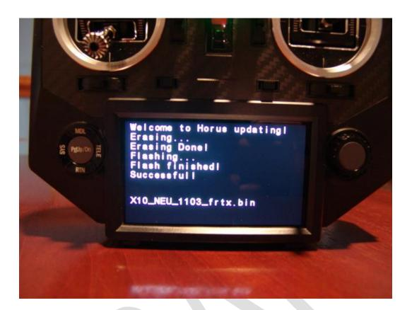
The firmware flashing process will run and finish with a "Successful" press the power off button briefly and the system shuts off.
