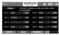
3. Failsafe can be set on receiver via short press Bind button while moving channel position to a preset value after binding.
