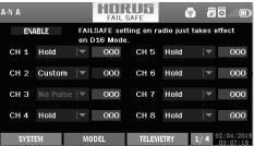
3. Failsafe can be set on receiver via short press Bind button while moving channel position to a preset value after binding.
