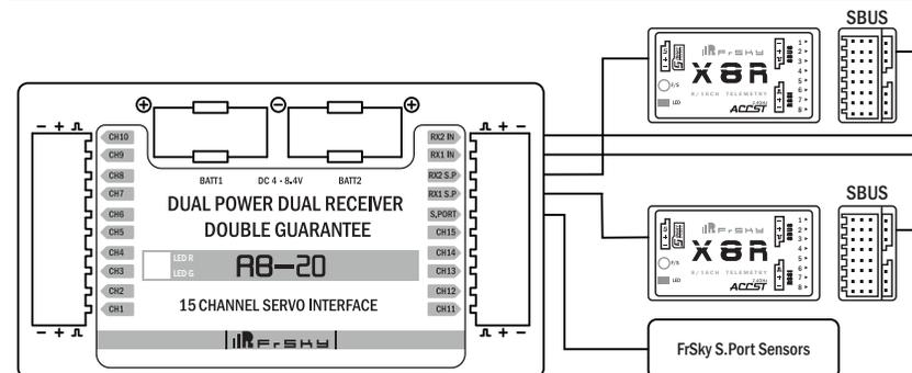
The RB-20 is a switchboard connected to power supplies, receivers, servos and S.Port sensors. The RB-20 does not contain circuitry to stabilize or regulate voltage to the servos. The level of the input voltage is equal to the level of (output) supplied voltage to the servos. Be sure to match the proper type of servos with your selected power supply (for example: when using 2 LiPo cells without a regulator, it is necessary to use servos labeled "High Voltage").
